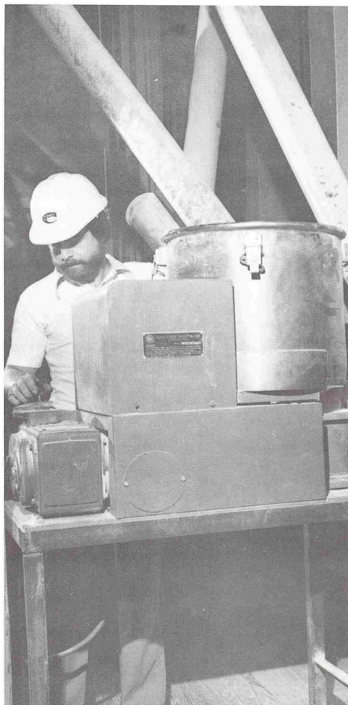
Controlled feeding is achieved as Mr. Lee Augustson sets regulator on Vibra Screw Live Bin Feeder.
