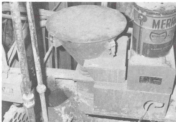
A high-purity micronized zinc powder is efficiently delivered by the Live Bin Feeder at DeLamar Silver Mine.
