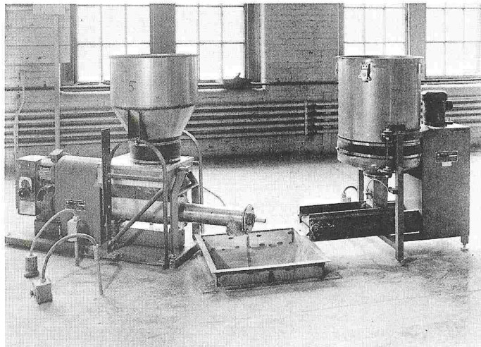
The blending of hot-melt resins with an antistatic compound has been accomplished by using a Vibra Screw Heavy Duty Screw Feeder (left), Volumetric Belt Feeder (right) and Vibra-Blender (not pictured) in combination. Both feeders deliver a continuous, accurate flow of material to the blender.
