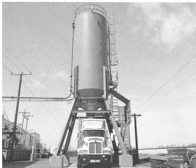
The Bin Activator can fill a trailer with 40,000 pounds of matted brass scrap in about two minutes.
