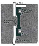
slippage. Stainless Steel clamps fit securely between the beads and tighten easily and effectively. This sleeve design is so effective it will withstand 10 psi internal pressure and is standard on all Bin Dischargers. Special compounds for high temperature and a flanged bolted sleeve for high pressure are also available.
