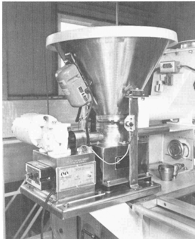
Newest pasta line at Zarega's Sons features two SCR-20 vibrating screw feeders completely fabricated of food-grade stainless steel.
