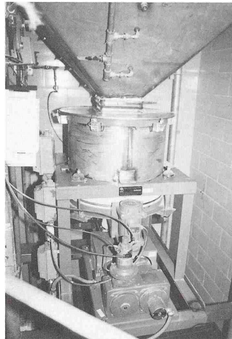
The Live Bottom Bin has a static hopper and movable Bin Activator, preventing segregation and providing first-in, first-out flow to the Live Bin Feeder.
