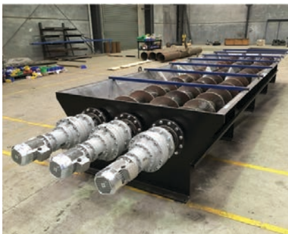
FIGURE 10. Live-bottom screw feeders are best employed in applications with large discharge openings. They employ several feed screws in tandem to prevent the formation of bridges or caverns in the material
