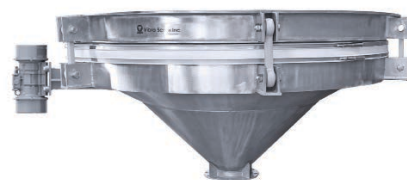
FIGURE 3. A bin activator replaces a portion of the bottom cone of a typical bin, providing vibratory action to encourage flow
