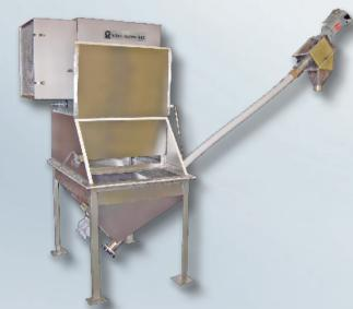
Bag Dump station with integral self contained dust collector
