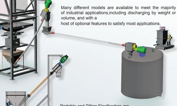
Portable and Tilting Flexifeeders are available with integral support stands.
