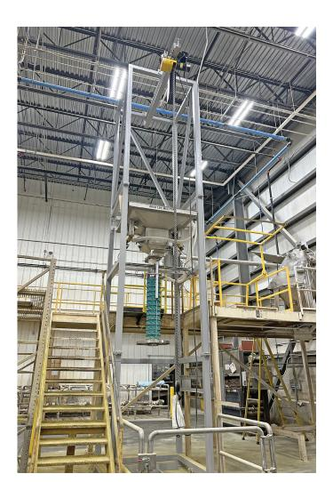
the Vibra Screw bulk bag unloader, only a single operator is required for the same daily volume. Although materials typically flow well into the bulk bag unloader most of the year,
