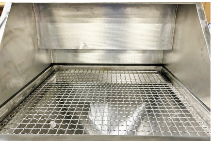
Internal safety grid facilitates the positioning of the sack and protects the downstream equipment from foreign objects.
