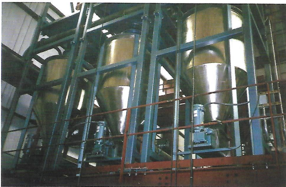
Three 6-inch-diameter volumetric screw feeders beneath the hoppers meter material to a 10-inch-diameter vibratory tube conveyor.
