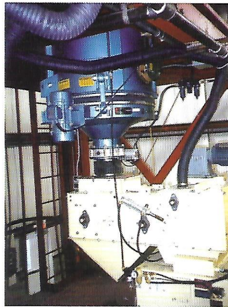
A live-bottom bin supplies packaging equipment.
