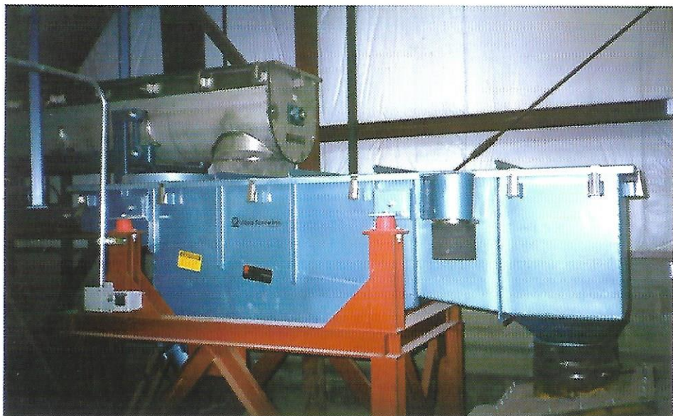
A continuous vibratory blender (top) discharges to a scalping screener (center).
