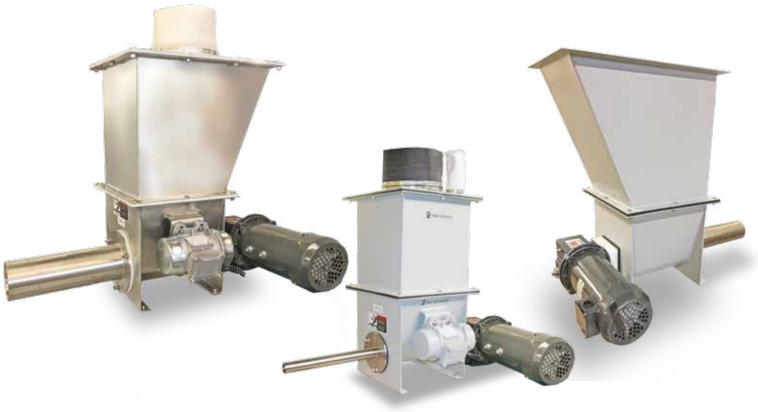
The **Model VSF-1 Volumetric Feeder** is a simpler, lower cost version of Vibra Screw's highly successful and proven Versifeeder. It has a foot mounted design with motor and gear reducer supported directly off the feeder trough. This eliminates the need for a separate support base and permits greater installation versatility with easy disassembly for cleaning. It retains the Versifeeder's popular modular design, enabling a single unit to adapt to the broadest range of feeding applications:
