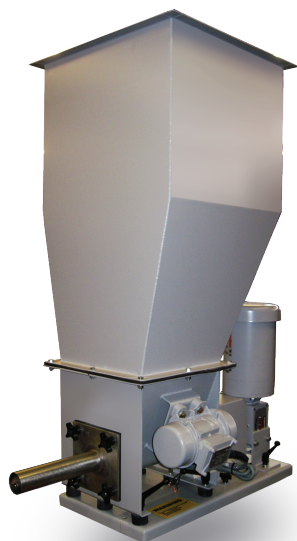
Standard VersiFeeder with 5 ft 3 hopper
