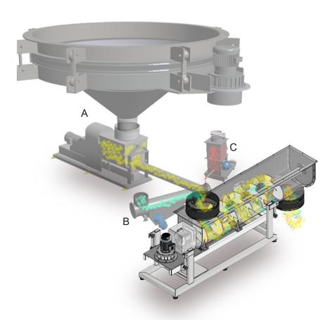
A) The patented Bin Activator attaches to new or existing storage bins and discharges materials in a positive, continuous flow. In the illustration, the Bin Activator discharges to a vibratiing Heavy Duty Screw Feeder, which delivers material to the blender at rates up to 10,000 ft<sup>3</sup>/hr with accuracy of  $\pm$  1-2%.
