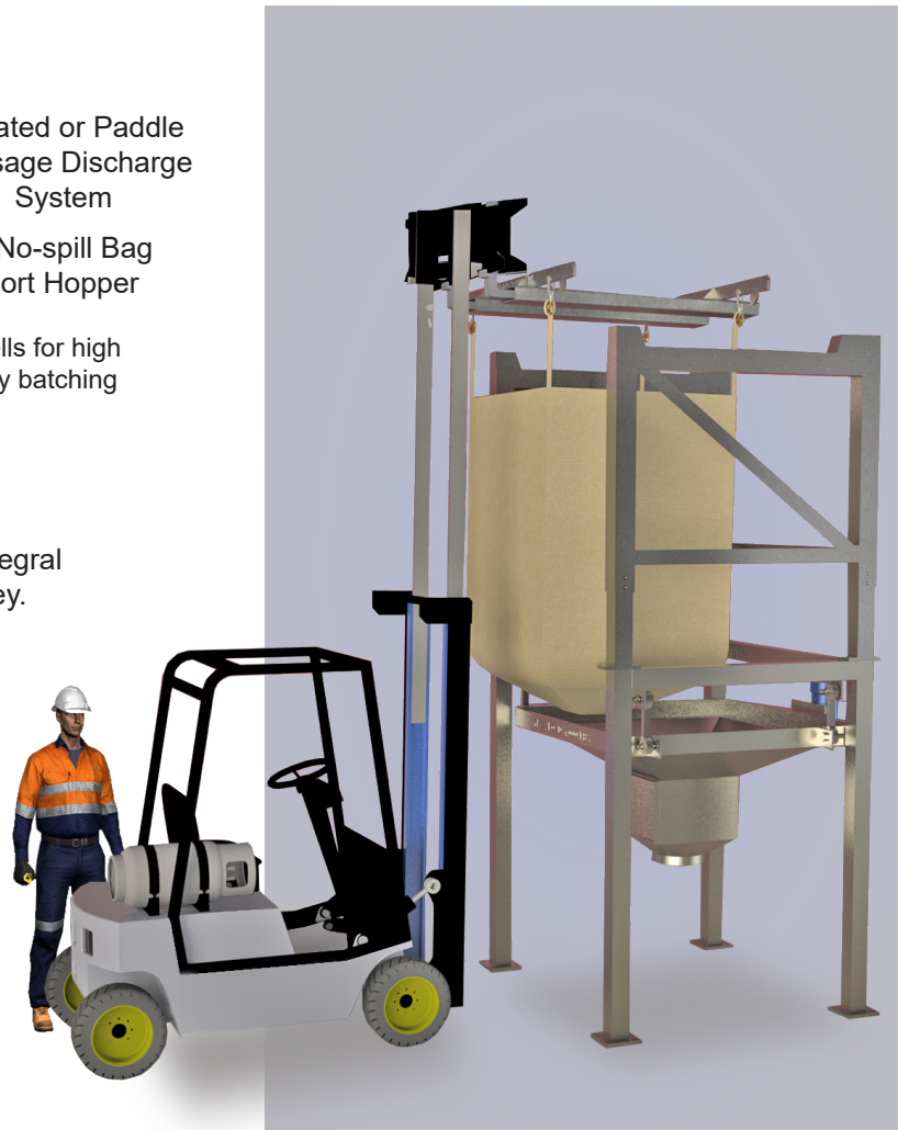
Model 2-VHD Fork-Lift Bag Rack An efficient fork lift compatible, bag lifting adapter and integral support frame allow operators to utilize lift trucks to place bags into position on the discharge hopper. Specify an adjustable height frame, and you can change the working height up to thirty percent, an important feature for variable size bags
