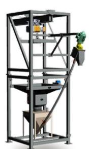
The use of controlled vibration at the inlet hopper eliminates material packing and tunneling and encourages more even loading of the conveying screw. This, along with a simple robust drive system, results in a more uniform repeatable conveying rate and dramatically reduces maintenance.
